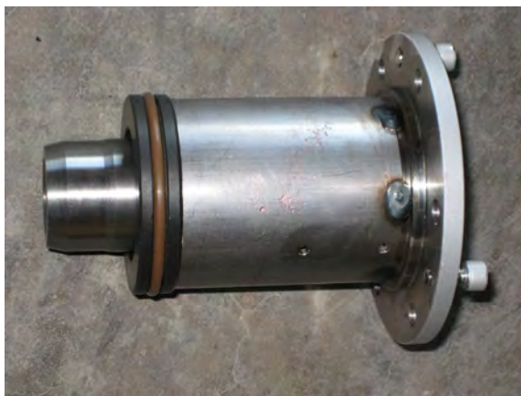
Rotary Seal Installed
