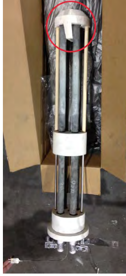
Pic.5 Hanger Bar+Lower Block+Spacers Pic.6 Adding Middle Block Pic.7 Adding Flange Pic.8 Heating Element Assy Pic.9 Braided connection
