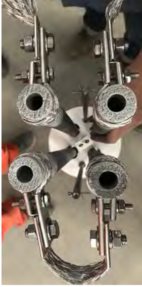
Pic.5 Hanger Bar+Lower Block+Spacers Pic.6 Adding Middle Block Pic.7 Adding Flange Pic.8 Heating Element Assy Pic.9 Braided connection
