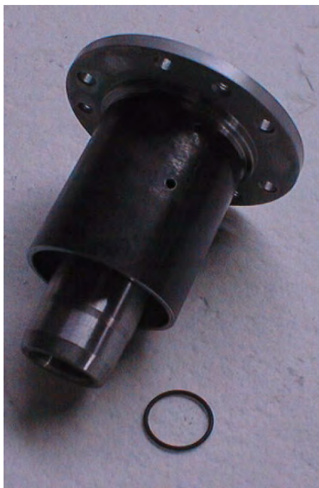
Bearing Package and typical "O"-Ring
