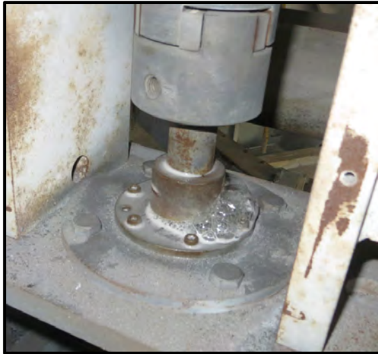
Leak Check at Bearing Package with leak spray
