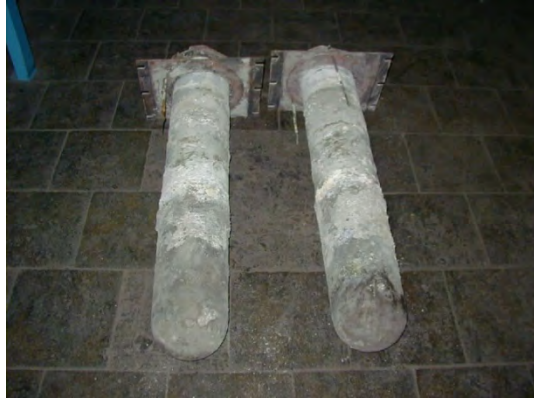
Pic.6 Sialon tubes removed from cover
