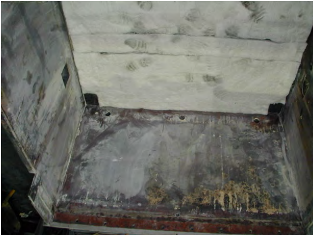
Steel shell interior with ceramic blanket on floor with square shims at corners
