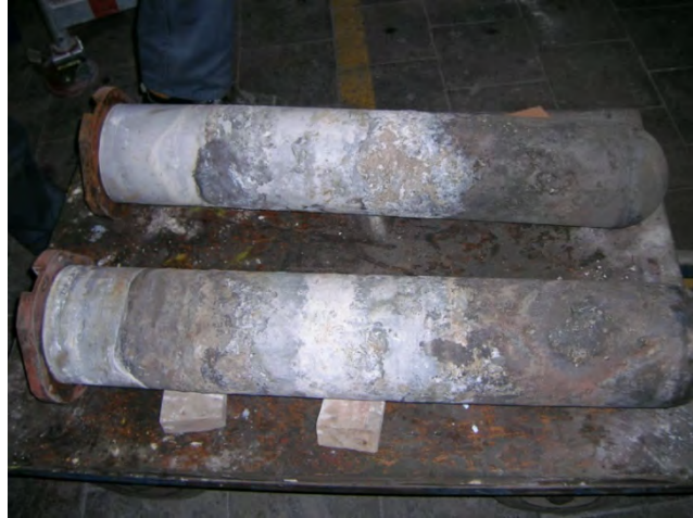
Pic.8 Sialon tubes after treatment
