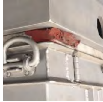
Picture 4. RTV sealant application
