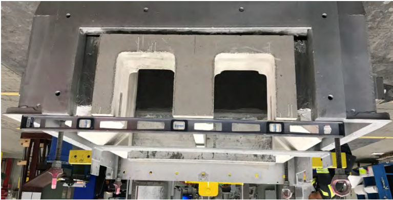
Centering the new cartridge in the steel shell
