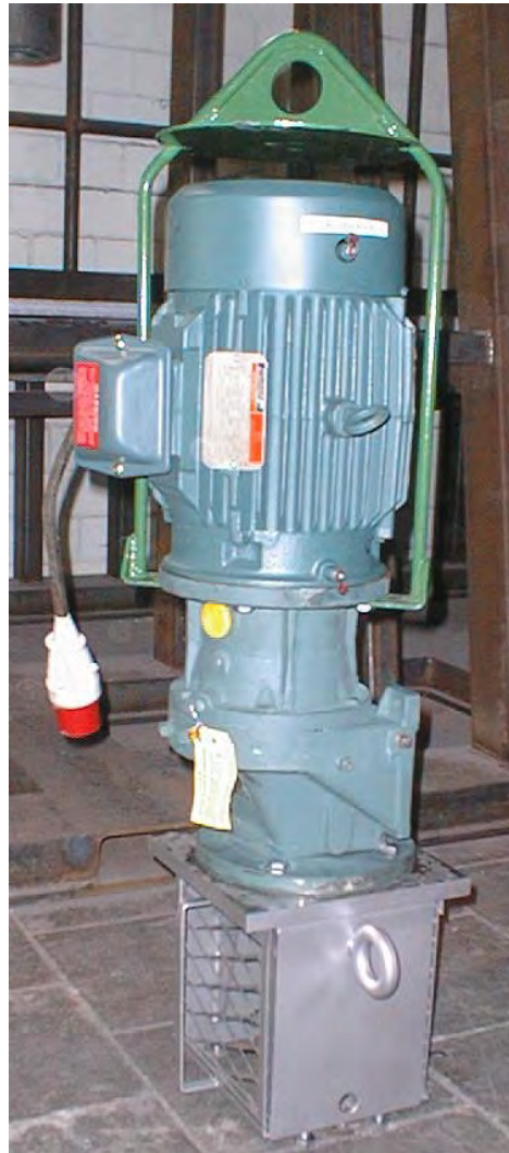
(b2) Motor Stand with Gear Reducer
