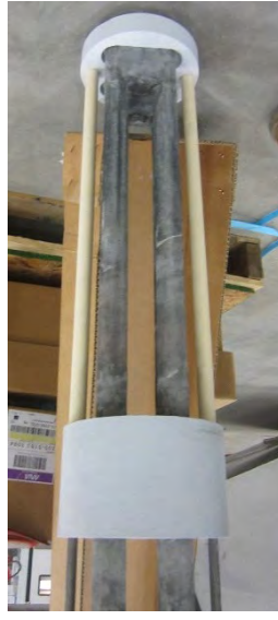
Pic.5 Hanger Bar+Lower Block+Spacers Pic.6 Adding Middle Block Pic.7 Adding Flange Pic.8 Heating Element Assy Pic.9 Braided connection
