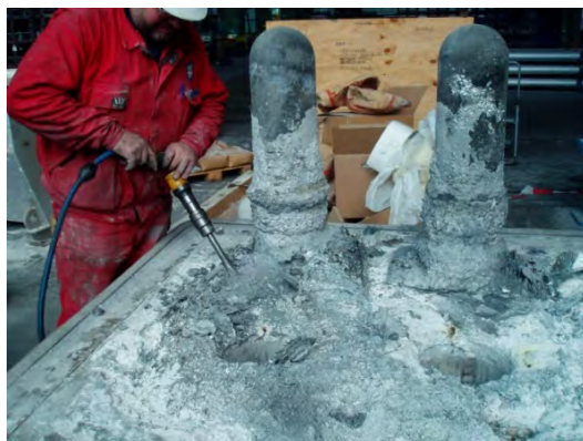
Pic.4 Remove build-up using pneumatic chisel
